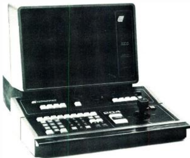
ESC-204 editor, with characteristic Convergence joystick.
