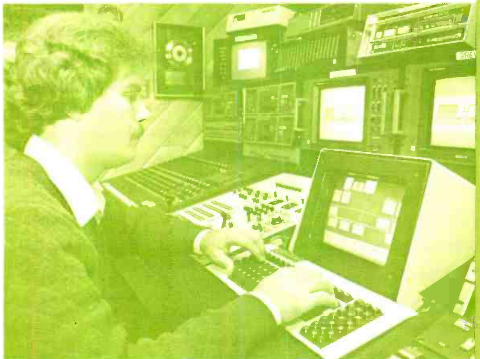
Bob Head at Henderson-Crowe's LightFinger Plus. Operator can interface system through screen, keyboard, or directly through tributaries (to right of program monitor).
